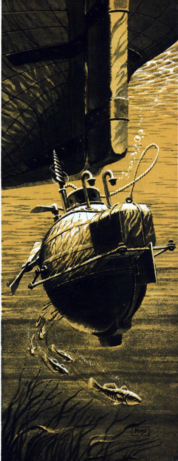
underwater range, would have to approach her target on the surface, probably at night to reduce chances of being sighted. He installed a compass and coated the main points and needle with a phosphorescent, decayed wood called foxfire. The depth-gauge float was similarly marked for visibility in total darkness—probably the first use of luminous instrument dials.
